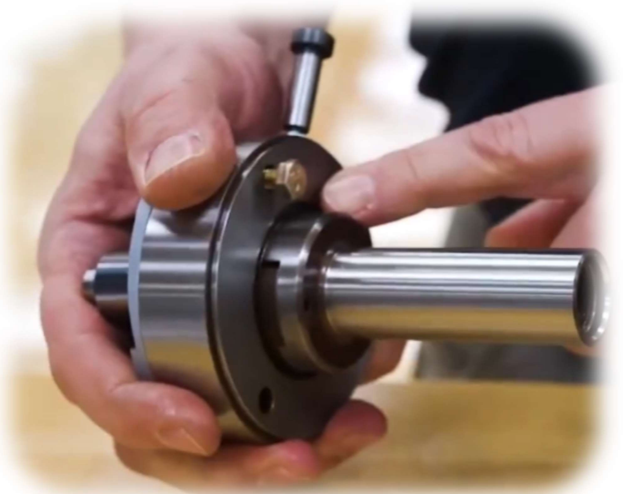
Fig. 23 – 191 ER attachment disassembled for periodic maintenance
